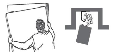
Adjust door height with screwdriver to clear carpets and align door with jambs
