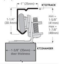
2 Hook door to track by tilting door until wheels slip into "V" section of track.
