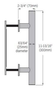
KT301SSH (PACKAGED IN BOX) Handle and flush pull, brushed ss, fits 1-3/8" (35mm) or 1-3/4 (44.45mm) door thickness. KT301BLACKH (PACKAGED IN BOX) Black Powder Coat KT301SSHR (CLEAR PACKAGING) Handle and flush pull, brushed ss, fits 1-3/8" (35mm) or 1-3/4" (44.45mm) door thickness. KT301BLACKHR (CLEAR PACKAGING) Black powder coat
